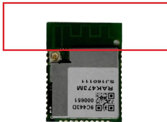
Figure 2-4 Clearance Schematic Diagram of PCB antenna area
