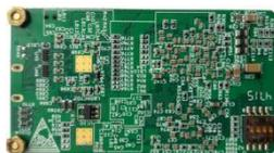
Notes : The DIP Switch is using for some new function . Must keep the lebel 3 and lebel 4 localing in OFF position.Or will make the module abnormal .
